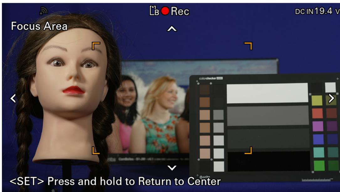
**Flexible Spot:** This is a much smaller area, useful for isolating a single object or very small part of the image. The flexible spot can be moved around the image using the thumbstick on the hand grip or the up/down/left/right menu button.
