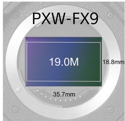
The Super 35mm modes use a smaller, central part of the sensor that is of a similar size to a frame of super 35mm movie film (S35). This is the same frame size as cameras such as the PXW-FS7 or FS5. In this mode you can use lenses designed for APS-C, S35mm, as well as lenses designed for Full Frame. In the S35 mode, if you use a Full Frame lens the field of view will be narrower than it would be in the Full Frame mode by a factor of 1.5.
