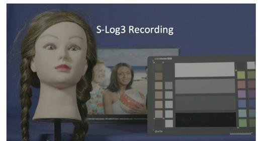
Exposure index is reduced to 200EI, image via the LUT becomes 2 stops darker
