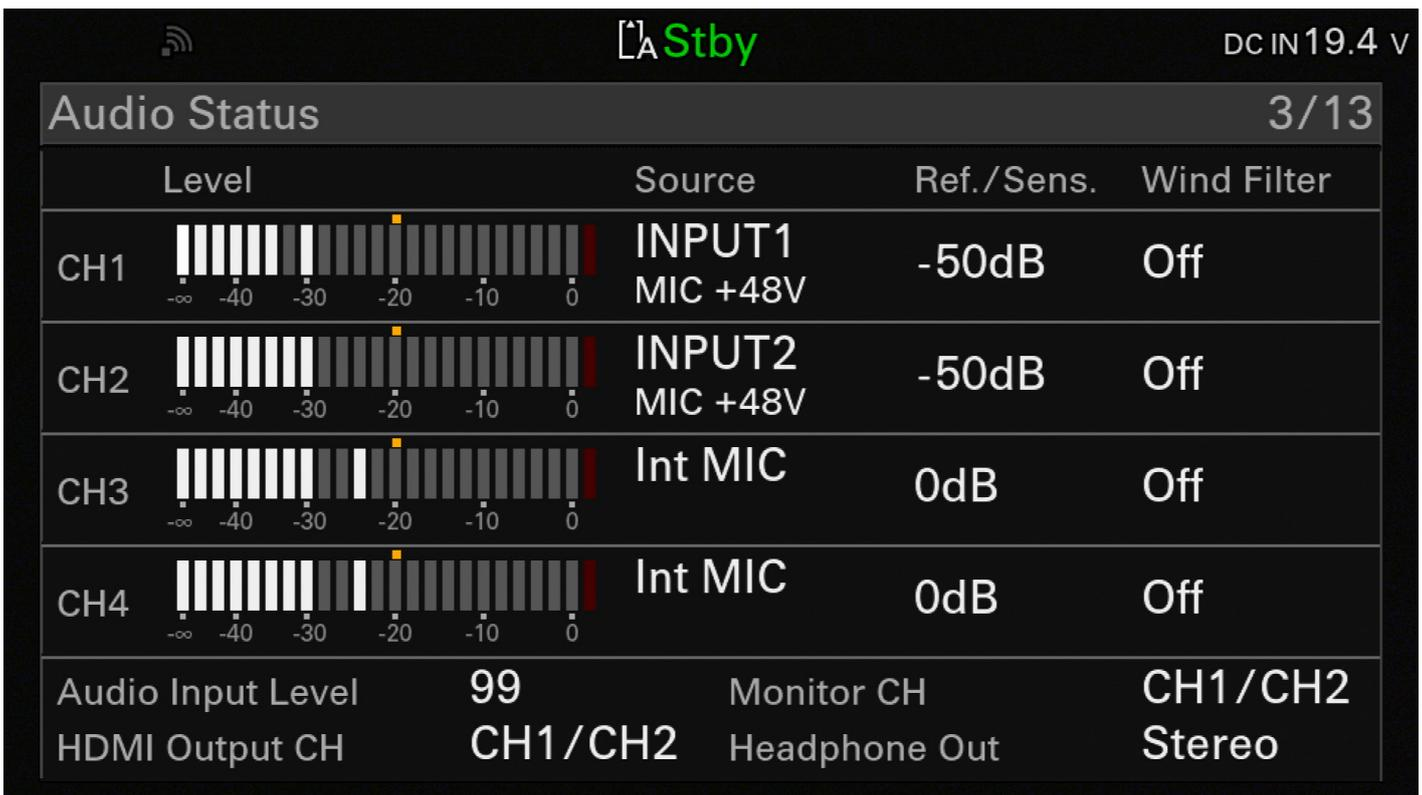
By going to **(MENU: Audio – Audio Output)** you can select which channels of audio are fed to the headphones. When the Headphone Out is set to mono the audio channels are mixed together. When set to Stereo and CH1/CH2 or CH3/CH4 selected each channel will be fed independently to the left and right headphone channels.
