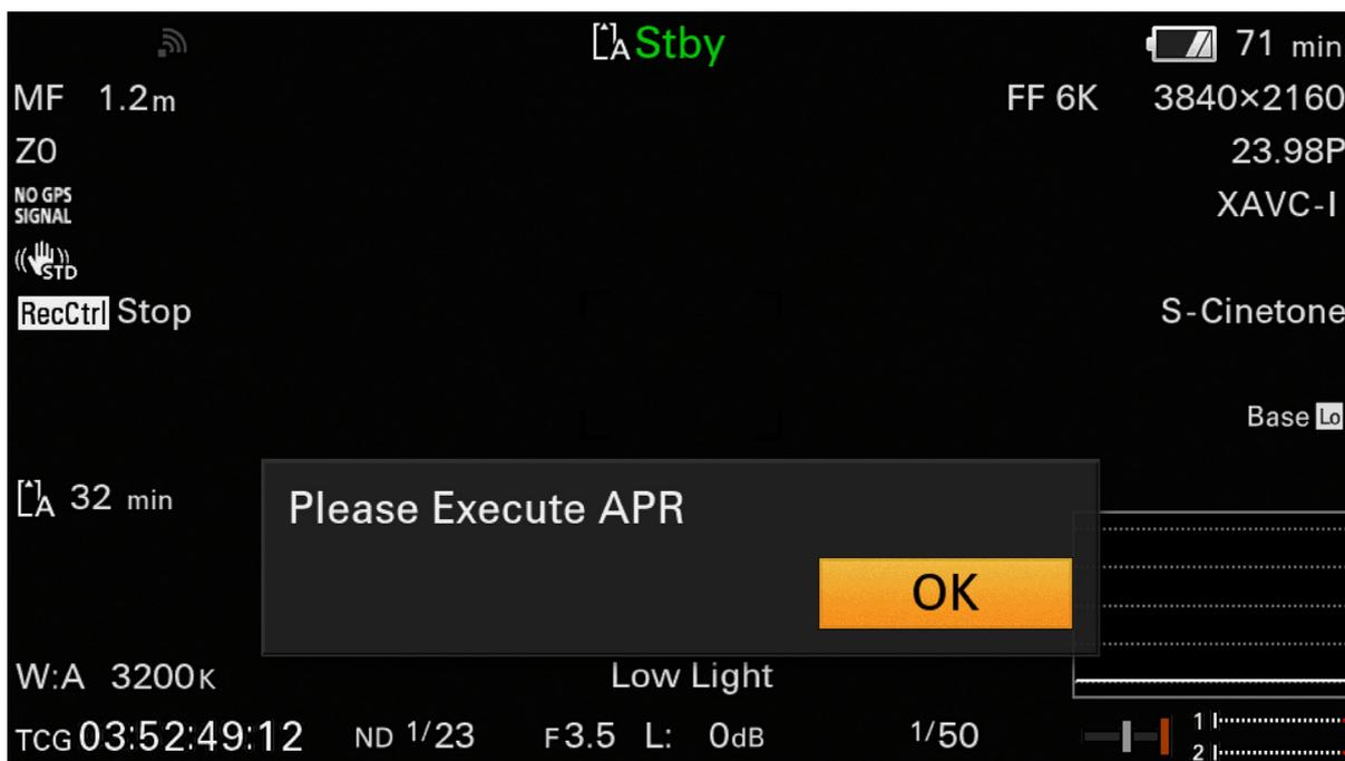
Cover/cap the lens so that all light is excluded and press the Multi-function Dial, the handgrip thumbstick or the set button to execute the APR function.
