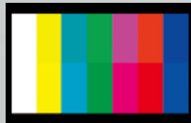
Color Space Comparison (Simulation): The top part shows the color space when set to the ITU-709 mode. The bottom part shows the color space in the WIDE3 (D-Cinema) mode. This screen image is simulated to show the differences in colors when using different modes.
