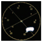
Fluorescent daylight full output (Gain x5) Note cyan color shift
