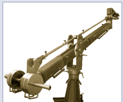
GF-8 in Jib Arm mode with counterweight rod
