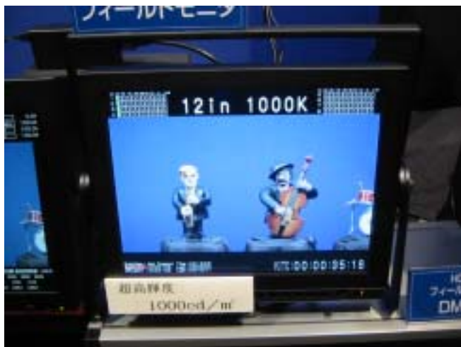
←12inch LCD monitor with ultra high brightness(1000cd/m 2 )
